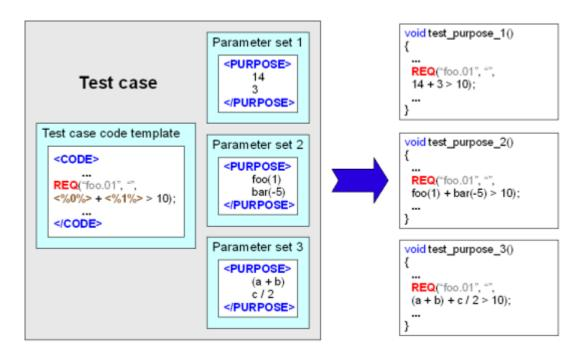
For each interface a test case template is created with a call of REQ macro for each requirement (see III.4.6.1). REQ is used to check the requirement and report failures. It receives a requirement ID, an expression to evaluate and some other data as its arguments. If the expression evaluates to 0, it means that the requirement (assertion) has failed. In this case the appropriate message is output to the TET journal along with the requirement text and the test result code is set to FAIL.
